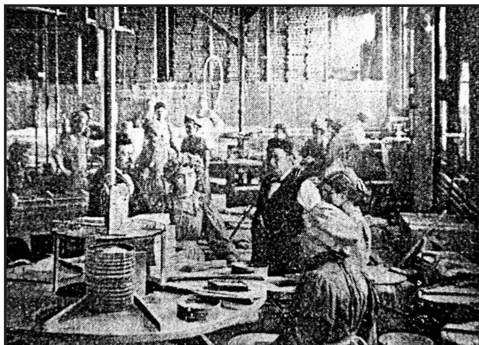
Fig. 4. Fabrication of Mueller encaustics. “Turning to the pressing room, our illustration shows in the foreground a circular bench, around which a number of young women are at work. The number of these depends upon the number of different colors in the tile. Each girl has her box of clay and her perforated card, by means of which she puts in her portion [color] of clay and then passes the frame to her neighbor. When it has made the round and all the divisions are filled, the frame passes to another operative [press operator] who lifts out the cell-frame, with a dexterous straight-up movement, leaving the little mosaics standing undisturbed side by side. The plain clay backing is then put on, the whole is put in the hydraulic press and the tile is ready or drying and burning.” Mueller and Langenbeck can be seen standing just behind the operatives and the circular table.
