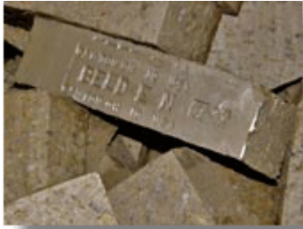
Every Belden brick is marked with the year it was made (07) and the clay formula used (42).
